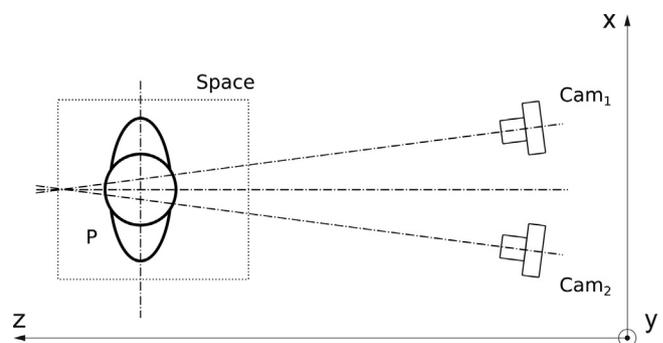
Fig. 1. Measurement set-up. Coordinates x, z as on the axes, y-axis is perpendicular to the drawing plane. Space – calibrated measuring space (as described in text), P – examined person under measurement, Cam<sub>1</sub>, Cam<sub>2</sub> – photogrammetric stereopair.
