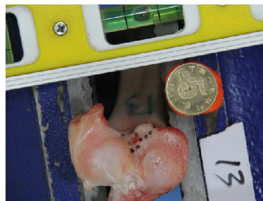
Fig. 2. An example digital image for the bundle insertion footprint surface area measurement. For scale calibration, a coin (diameter = 20 mm) was placed next to the footprint with the coin positioned in the same plane with the footprint, verified with a level. The image was also marked with the sample number (knee #13 in the example).
